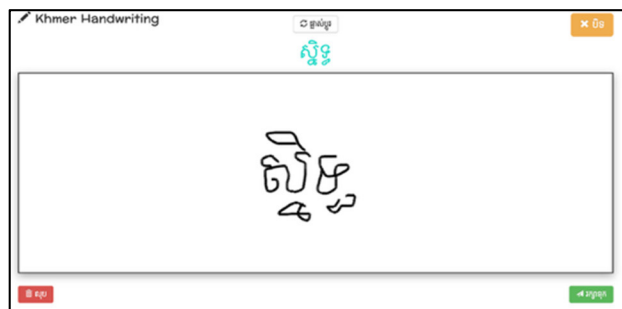
FIGURE 9. User interface for drawing Khmer scripts using OTKH. The black word (រូប) represents the user's handwritten input, while the blue word above represents the word generated from the database (photograph by author). The word drawn by the user is represented as a series of points (x,y).
