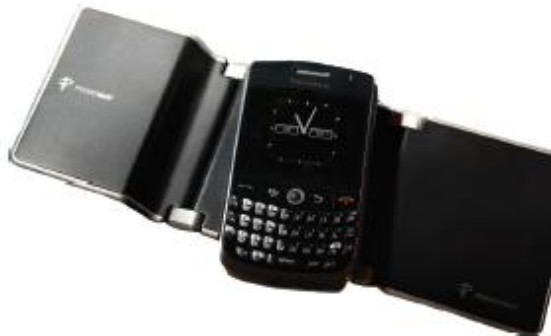
Figure 5-25 Wireless charging platform
